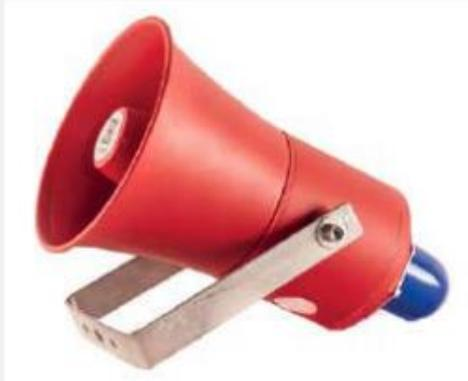
The flameproof ZT-SB150-1 sounder and beacon combination is ATEX / IECEx certified for use in potentially explosive atmospheres and provides clear visual and audible status indication (can be labelled accordingly). It is constructed from GRP.
