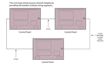
Two core loop wiring ensures network integrity by providing full isolation of faulty wiring segments.
