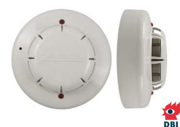
The Fyreye Extra analogue addressable optical smoke detector is particularly suitable for detecting optically dense smoke, involving materials such as soft furnishings, PVC, plastic, foam and all similar materials which produce small visible particles (0.5 to 10 µm).
