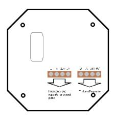
Two terminal blocks are provided on the back of the PCB to facilitate the installation of multiple repeaters. The panel can be connected to either of these terminal blocks.
