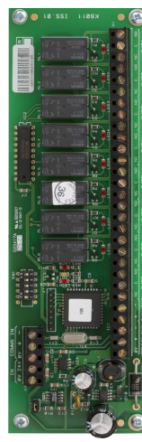
8 Way Relay Extender Board (K547)
