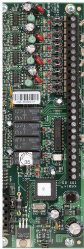
4 Way Conventional Detection Zone Module (K545)
